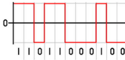
A typical NRZ coded signal is implicitly filtered with a sinc filter.
