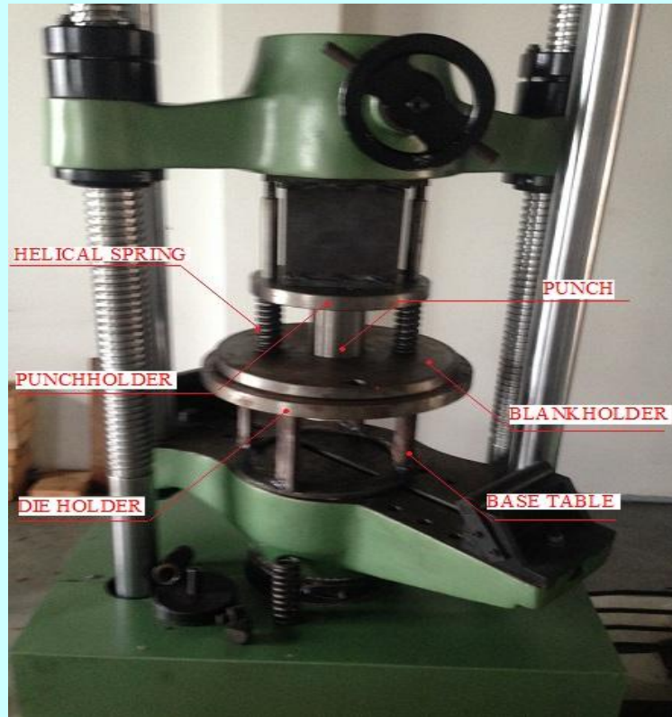
Fig: Close view of Deep Draw Die mounted on UTM
