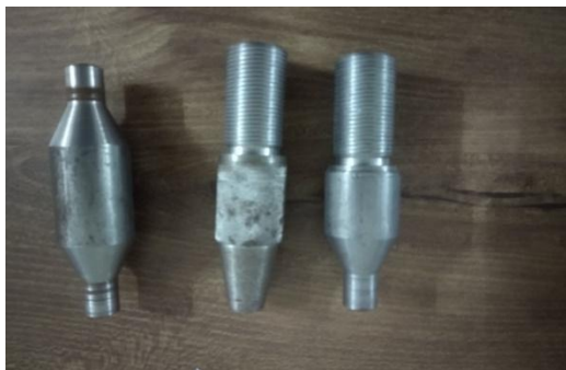
Fig:7 Knurling Operation
